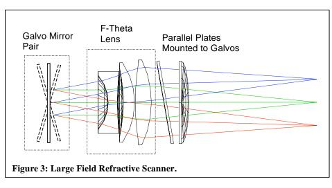
conventional galvo. The beam exits the F-theta lens of a conventional galvo scanner and passes through a pair of parallel plates, each of which is mounted to a galvanometer. The parallel plate
