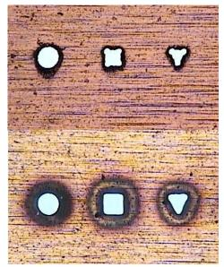
Figure 6: Conventional & NeoScan Scanner Machined Geometrical Shapes in SS
