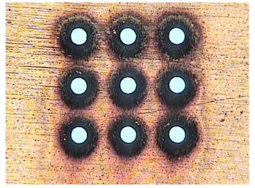
Figure 4: NeoScan Drilled Hole Array in Stainless Steel
