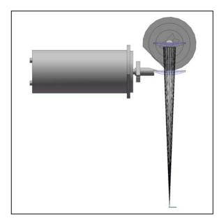
Figure 1: NeoScan refractive scanner with a pair of meniscus lenses mounted to galvos.
