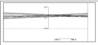
Figure 2: Enlarge view of ray trace of laser spot refracted away from the optical axis (dimensions in mm) Fig. 2 depicts an enlarged ray trace at the focal point of the lens system on how the light is deviated from the optical axis from the corresponding tilt of first meniscus lens in the X plane in Fig. 1.
